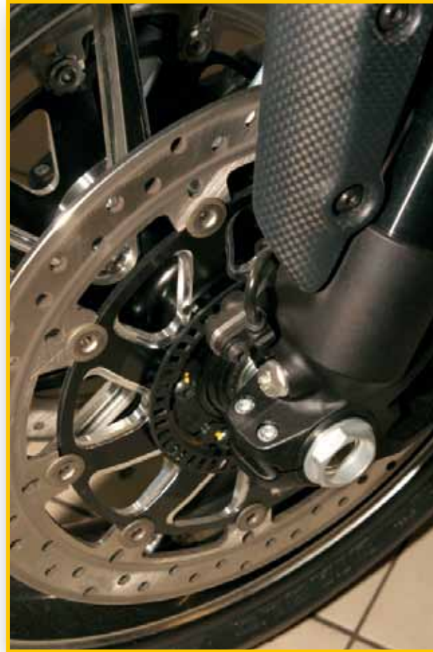
A typical ABS wheel speed sensor arrangement.
