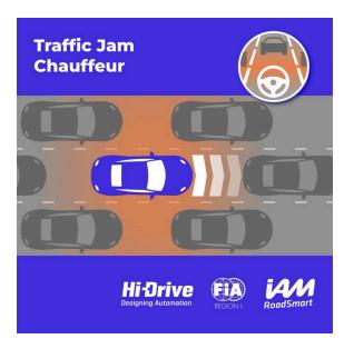
Traffic jam chauffeur (SAE level 2) monitors the speed of surrounding vehicles in slower environments of up to 60km/h.
