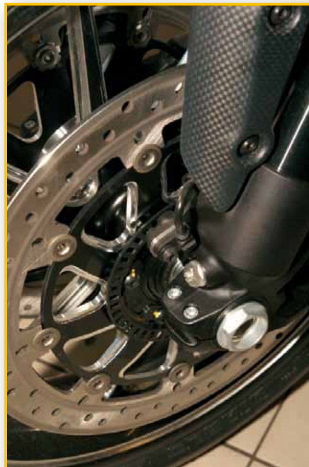
A typical ABS wheel speed sensor arrangement.
